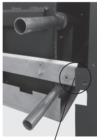
Right hand M6 bolt undone and side panel 'spread' for access
