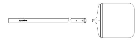
You will notice the handle end has an angle cut that matches the angled profile of the pizza peel end. Fit the stainless-steel end to the aluminum handle ensuring the angled end of the handle aligns to suit the pizza peel fold form. Line up the holes and use the 2x M6x12mm stainless dome head socket screws with 1 washer under each bolt head. Insert bolts and tighten.
